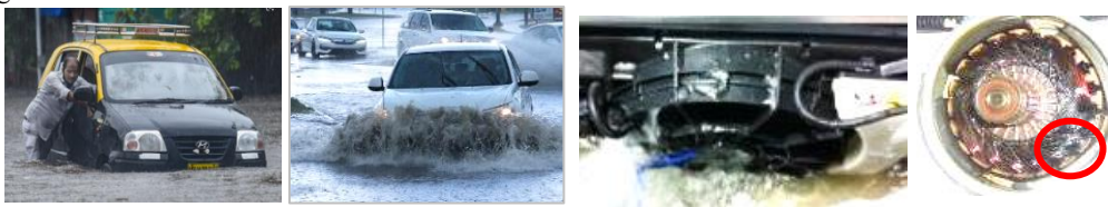
Fig.1 Flooded conditions and motor damage (disconnection)
