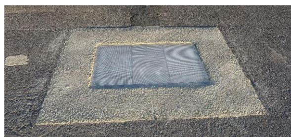
Fig. 3 Flush-mounted transmitter coil.
